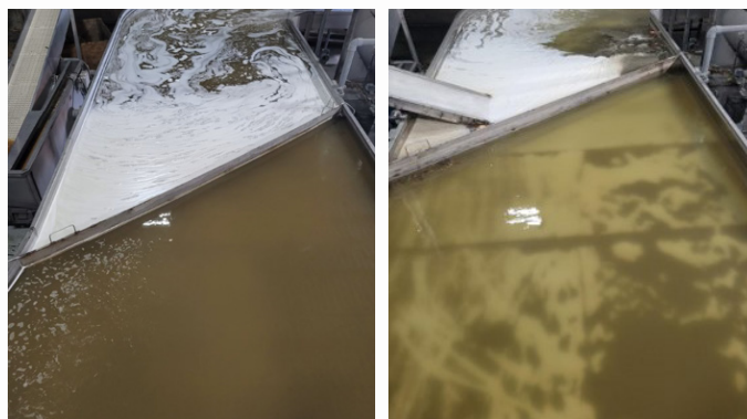
Flume water before and after enriching with oxygen and ozone nanobubbles shows clarity improvements.
